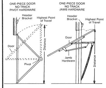
Locate height for header bracket by opening door to highest point of travel as shown. Measure distance from top of door to floor. Subtract actual height of door. Add 8" to the remainder. See example below.
